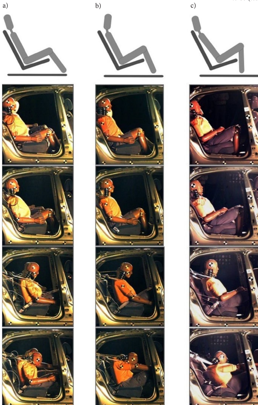
Fig. 1. A diagram of the initial dummy position and its view in the tests 2P (a), 3P (b) and 11P (c) in time t=0 ms, 40 ms, 80 ms and 120 ms
