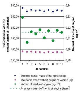
Fig. 3. Results of repeated measurement of inertial mass and moment of inertia of engine
