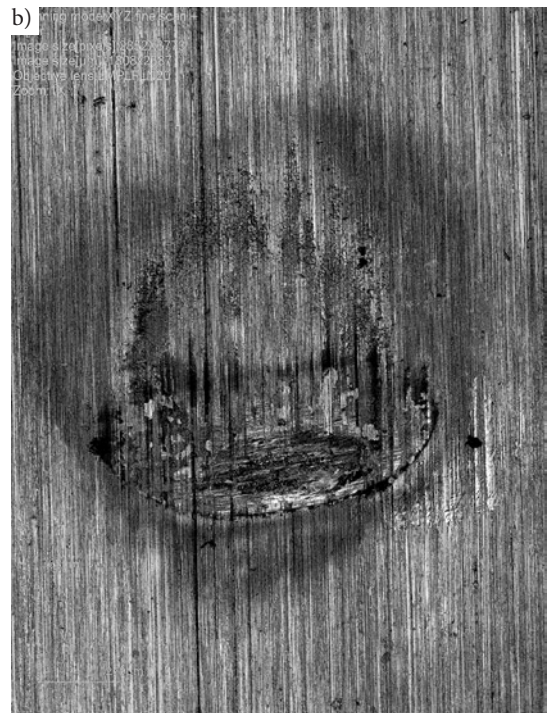
Fig. 8. Microscope photographs of the surfaces of 316L implantation steel samples after tests in the saliva environment: a) after fretting (SEM), b) after fretting corrosion (confocal microscope)
