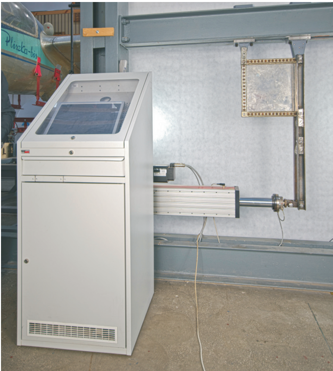
Fig. 5. A set-up for static and fatigue tests with a model made of aluminium alloy plate
