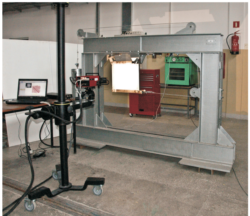
Fig. 2. The set-up for static experiments with 3D ATOS scanner
